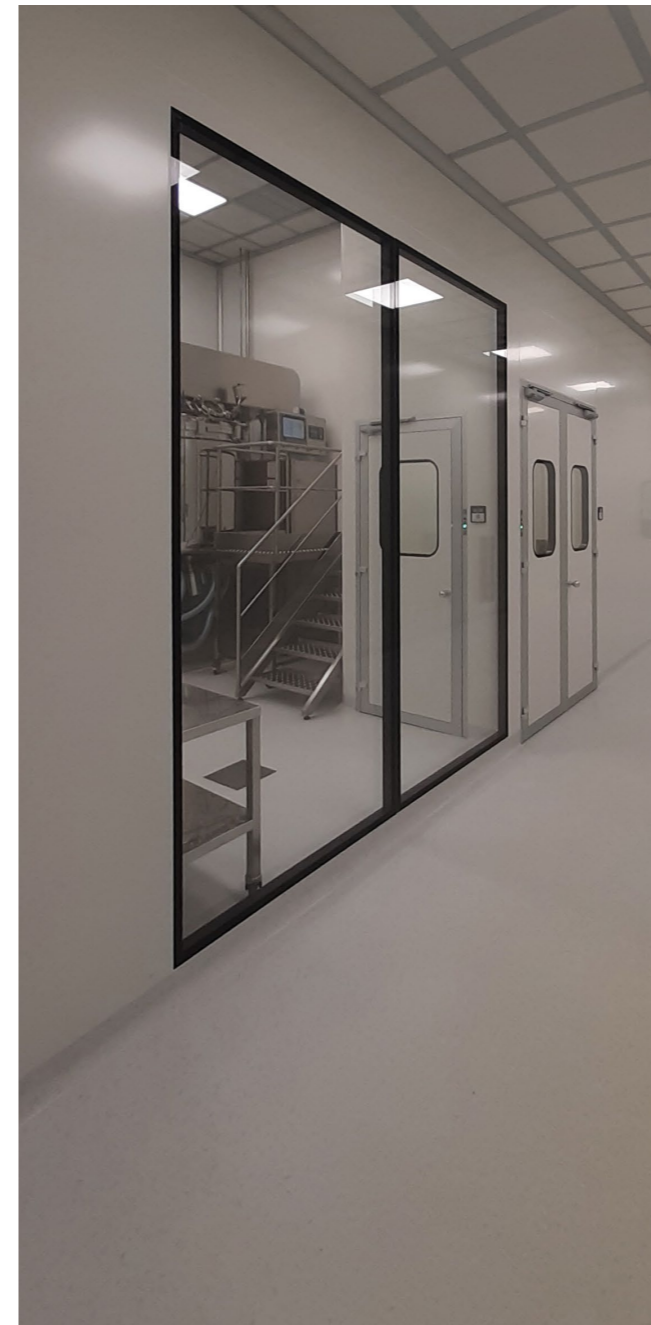
Parete serie 62 in alluminio preverniciato e visive a grande altezza / 62 series partition in pre-painted aluminum and high-height windows / Cloison série 62 en aluminium pré-peint et visuels de grande hauteur
